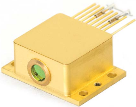
HHL package suitable for higher dissipation CW-DFB
